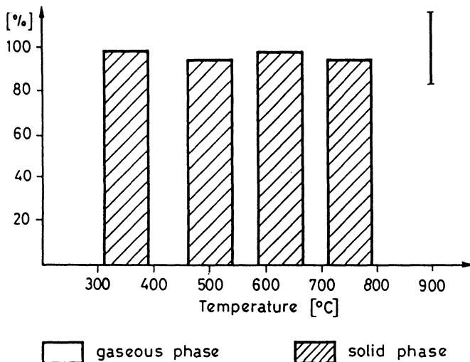
Figur 3: Distribution of Cr, Ni, Cu, Zn and Pb between gaseous and solid phase
